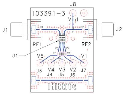
\* R2 - R6= 100 Ohm. These resistors are optional and may be used to enhance decoupling of the RF path from the control inputs.
